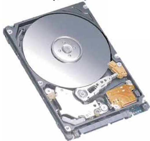
The disc of the hard drive moves from 5400 to 7200 times in a minute!
