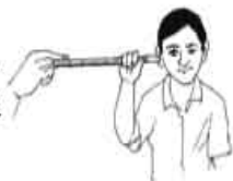
Fig- 8.6 : Circulation of Sound through solid substances
